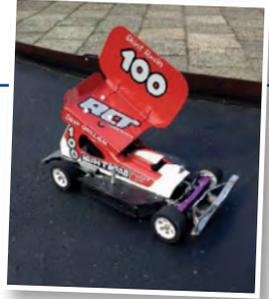
Cars are put together by drivers using a steel chassis frame, RC steering & throttle servos and nitro fuelled single cylinder 3.5cc engines provide the power, which is delivered to the rear wheels by a belt driven single beam axle.
