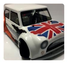
If it comes in the Kit its legal with a few additions. Servos cost £10, a G2 silver can motor slightly less, and 15/48 is the fixed gear ratio that levels out speeds in the class. Minis are run indoors so are a great all-year-round class.
