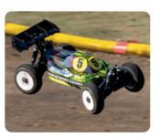
Our 1/8th Electric buggies are very similar to their Rallycross nitro buggy cousins but are electric powered, with 4s lipo batteries (or 2x 2s lipo's) replacing the nitro fuel to power the ESC (electronic speed controller) which controls the power to an electric motor (1900Kv to 2100Kv our most popular motors) replacing the fuelled engine.
