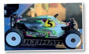
The cars that are raced are all four wheel drive powered by a 3.5cc nitro fuelled engine with double disc brakes to bring them to a halt. All feature fully independent suspension, which is adjustable to suit the driver and track conditions. With different spring tension rates, damper settings, antirollbars settings, and adjustable suspension geometry to fine-tune the car's handling. Different tyre patterns and compounds complete the set-up.
