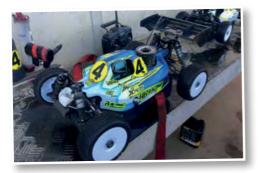
The cars that are raced are all four wheel drive powered by a 3.5cc nitro fuelled engine with double disc brakes to bring them to a halt. All feature fully independent suspension, which is adjustable to suit the driver and track conditions. With different spring tension rates, damper settings, anti-rollbars settings, and adjustable suspension geometry to fine-tune the car's handling. Different tyre patterns and compounds complete the set-up.
