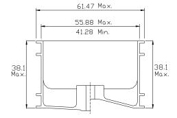
'Venting' holes in the internal rim of the wheel are allowed – maximum of two (2) holes, of maximum 6.0mm. diameter.
